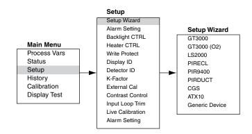
After selecting the type of detector, the SETUP WIZARD leads the user though the following selections:
