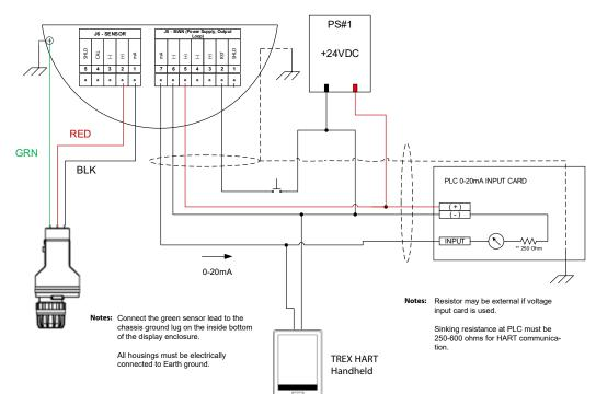
Figure 9 – UD30 with GT3000 Power Supply Voltage
