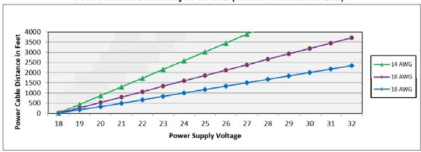
Recommended maximum cable from the power source to the UD30 is 2000 feet or 609.9 meters. Recommended maximum cable length from the UD30 to the sensor is 500 feet or 152 meters for 16 AWG wire.
