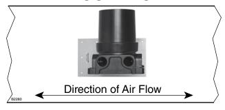
Figure 29 – Orientation of PIRDUCT Mounting Plate Relative to Direction of Airflow through Duct
