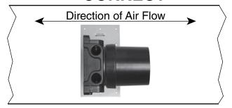
IMPORTANT: MOUNTING PLATE **MUST** BE ORIENTED AS SHOWN.
