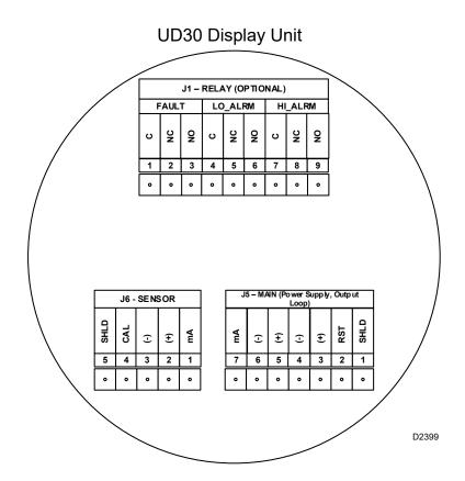
Figure 6—Wiring Terminals on UD30 Display Module
