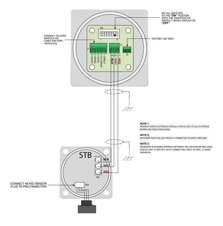
Figure 40 – CGS Wired Directly to the STB Sensor Termination Box
