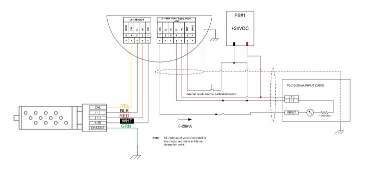
Figure 16 - PIR9400 Wired Directly to UD30
