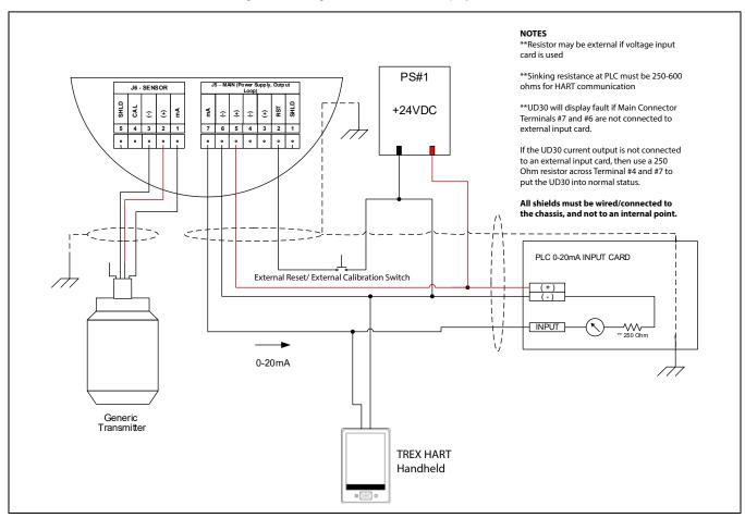
Figure 7—UD30 Wired to PLC using 3-Wire Shielded Cable with 0-20 mA Non-Isolated Sourcing Output
