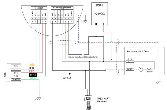
Figure 26 – UD30 with PIRDUCT Power Supply Voltage
