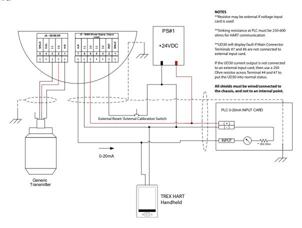
Figure 8 – HART Handheld Communicator Connected to the UD30's 4-20 mA Output
